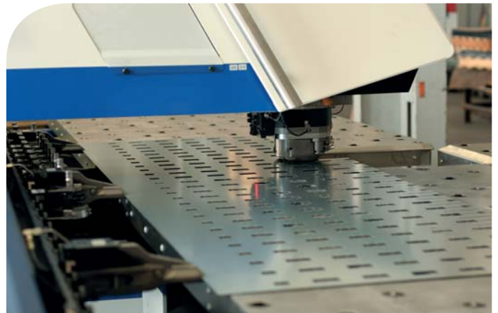
TopSolid'Sheetmetal offers machining strategies for each tool to optimize the path of the punching head on the sheet
